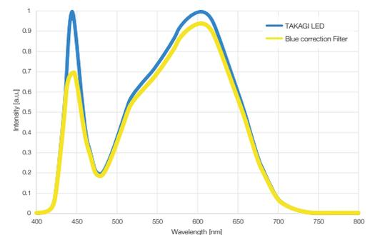
The 700GL is equipped with a blue correction filter that produces a colour tone similar to that of a halogen lamp, while preventing blue light-induced damage. Also, by using the blue cut filter to block blue wave lengths, it is possible to provide a light that is even safer for the retina.
